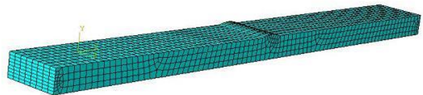
Fig. 8 Free meshing with linear tetrahedral and hexahedra elements
