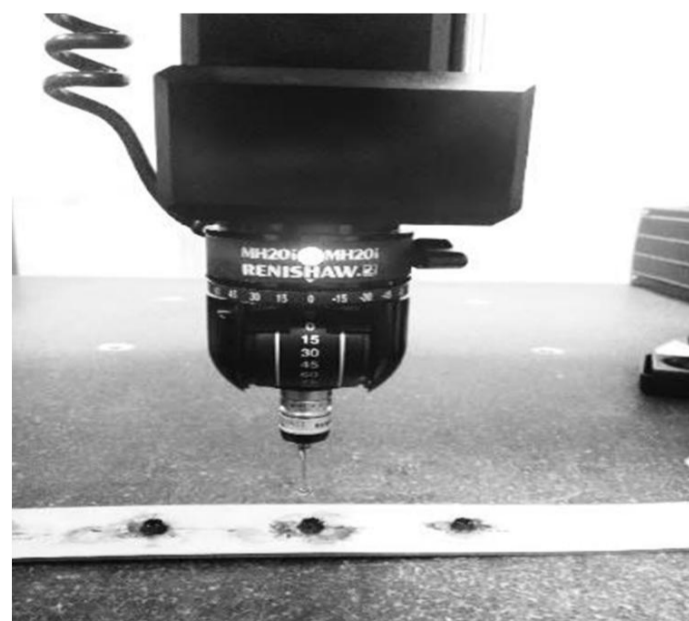
Fig. 6 Measurement of bush length by CMM
