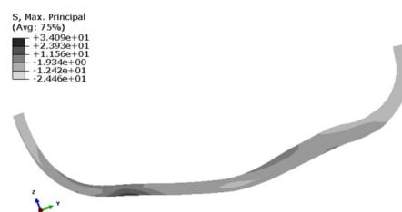
Fig. 11 Maximum principal stress distribution in the femoral cartilage through the thickness (MPa)
