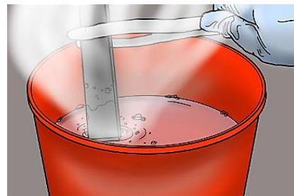
Fig. 1 The water tank for cooling in quenching process [22]
