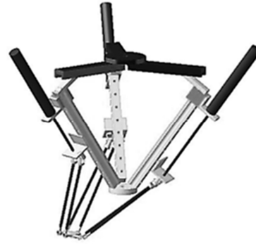
Fig.1 Schematic of a 3[P2(US)] parallel manipulator
