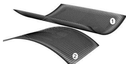
Fig.12 Simulation of the bistable composites 1)Steady state around the longitudinal axis 2) Steady state around the transverse axis
