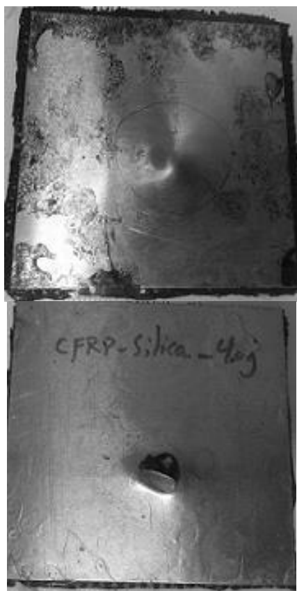
Fig.11 Aluminum back face damage a) with MWCNT b) with nano silica
