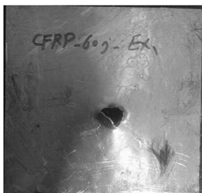
Fig.6 Comparison samples with 2-1 lay-up under 60j impact energy
