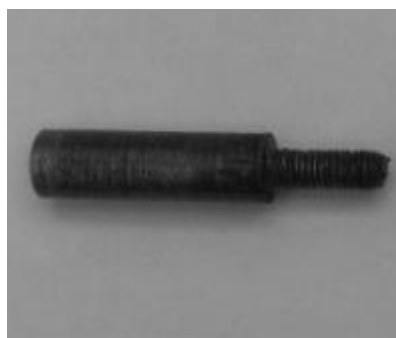
Fig.4 Projectile of blunt cylinder
