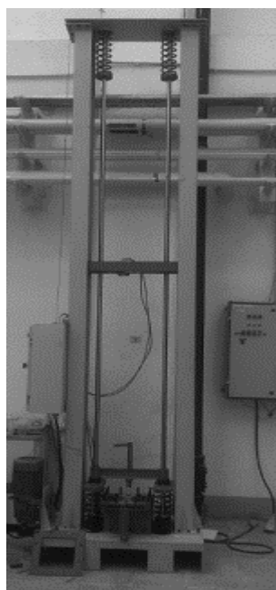
Fig.3 Low velocity impact device
