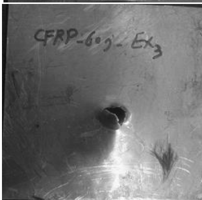
Fig.7 Comparison samples with 2-1 lay-up under 60j impact energy
