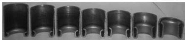
Fig. 7 Internally inverted sectioned tubes at different velocities (respectively from left to right, v=71, 81, 89, 97, 104, 110.5 & 126.5 m/s)
