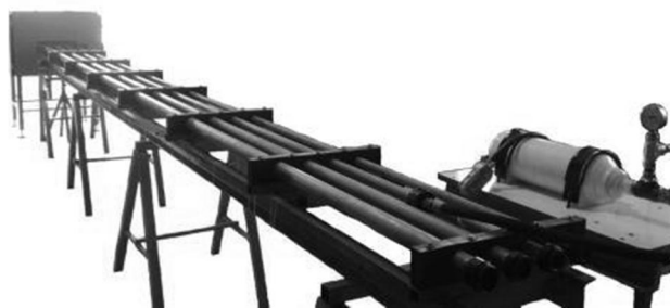
Fig. 1 Total view of Gas Gun
