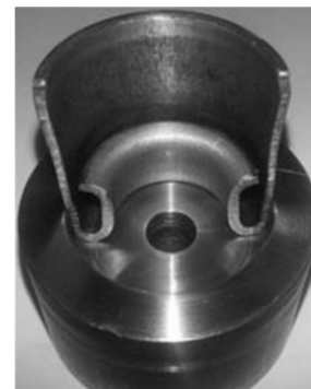
Fig. 6 Sectioned invertube on its respective die
