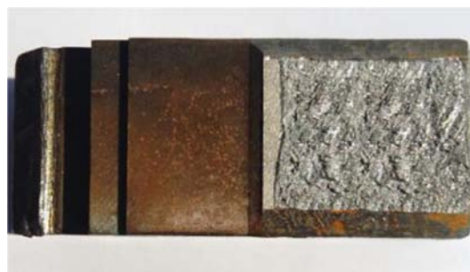
Fig. 9 Fatigue and fracture surface of CT specimen
