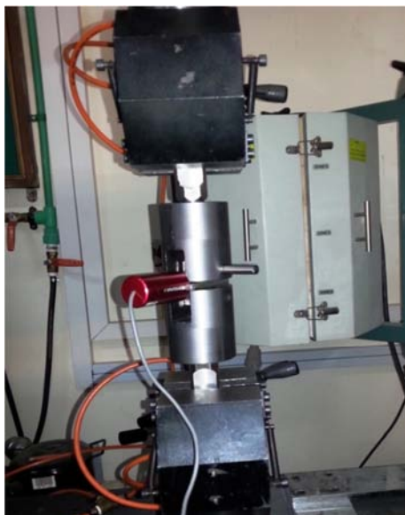
Fig. 7 Photograph of unloading compliance test equipment
