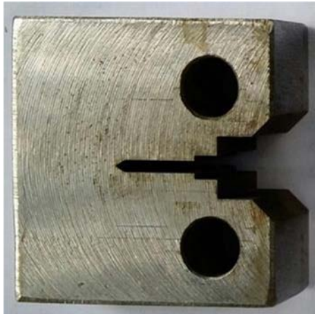
Fig. 5 Photograph of a machined CT specimen
