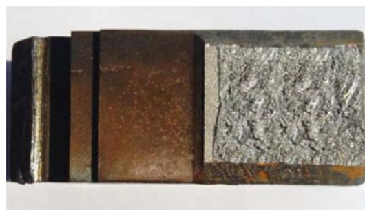
Fig. 9 Fatigue and fracture surface of CT specimen
