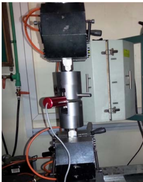
Fig. 7 Photograph of unloading compliance test equipment
