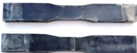
Fig. 4 Photograph of tensile test specimens
