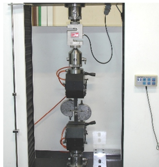
Fig. 5 The fracture test setup in the case of mode III
