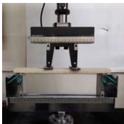
Fig. 4 Fixture loading for four point test
