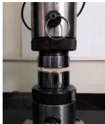
Fig. 1 Fixture of pressure test
