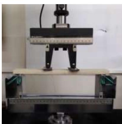
Fig. 4 Fixture loading for four point test
