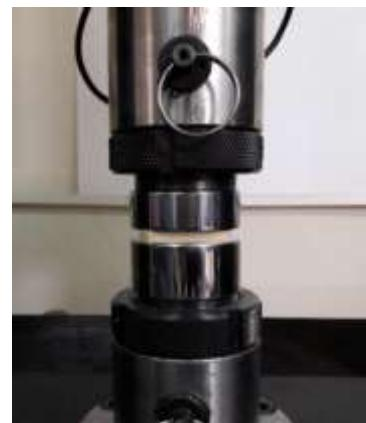
Fig. 1 Fixture of pressure test
