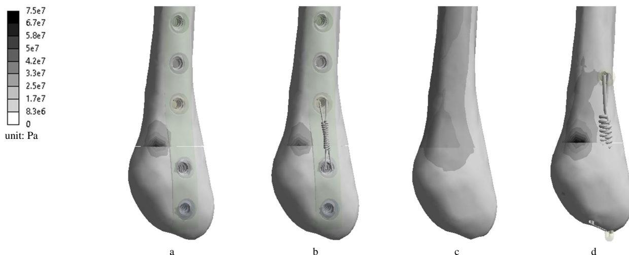
Fig. 10 Stress at the fibula under axial bending load: a) First technique, b) Second technique, c) Third technique and d) Forth technique
