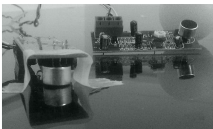
Fig. 3 Method of sensor attachment to a plate surface
