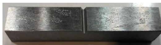
Fig. 8 Impact test sample according to ASTM E 23.
