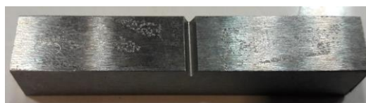
Fig. 8 Impact test sample according to ASTM E 23.
