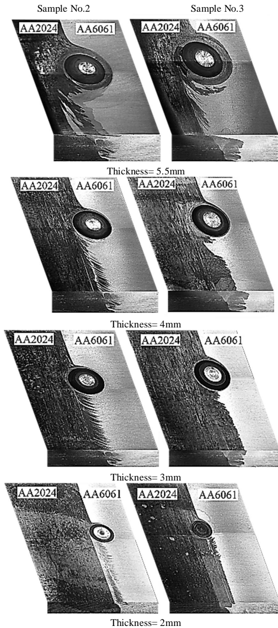
Fig.6 3D Cross-section macrostructure of welded samples at different thickness
