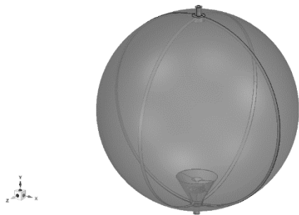
Fig. 15 Final tank and PMD schematic
