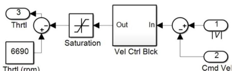
Fig. 7 Velocity Control sub-system for the simulated MAV
