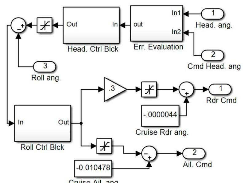
Fig. 12 Heading Control sub-system for the simulated MAV
