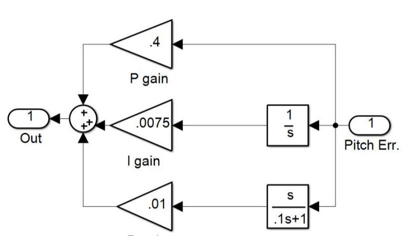
Fig. 11 Pitch Control Block
