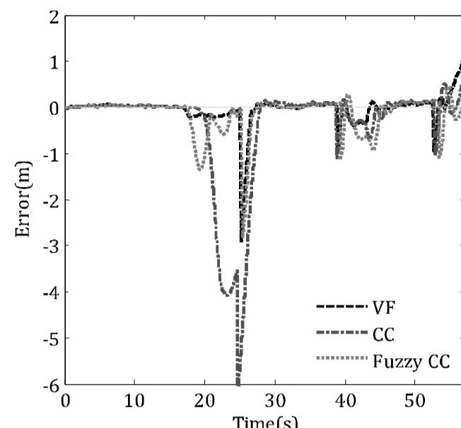
Fig. 27 Height error with applying wind disturbance
