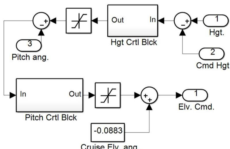
Fig. 9 Height Control sub-system for the simulated MAV
