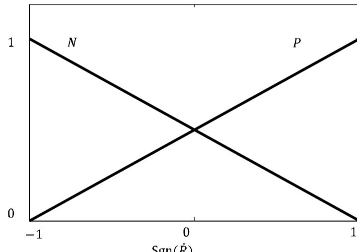
Fig. 21 Membership functions of the sign of  $\dot{R}$
