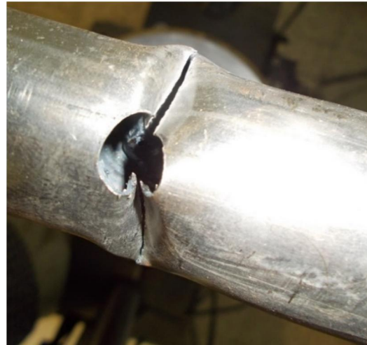
Fig.12 failure of specimen from location of cutout
