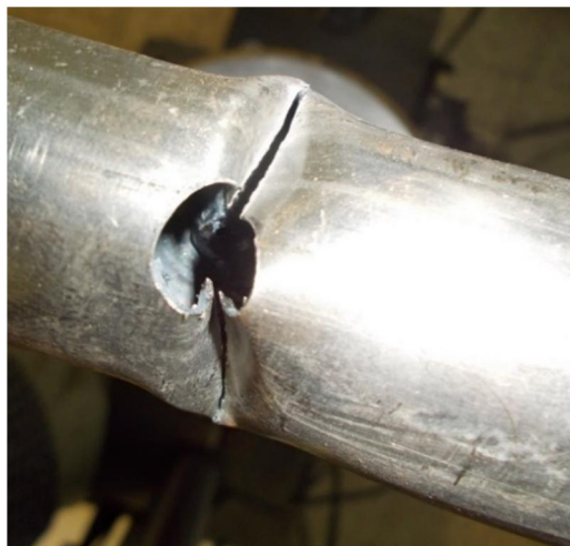
Fig.12 failure of specimen from location of cutout
