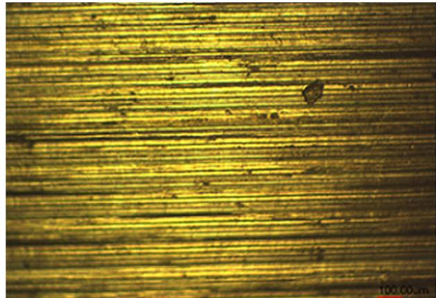
**Fig. 17** Developed image with an optical microscope of the workpiece surface under MQL
