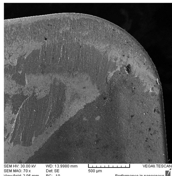
**Fig. 8** SEM image of rake face of tool under wet lubrication (cutting speed 70 m/min, feed rate 0.32 rev/min)
