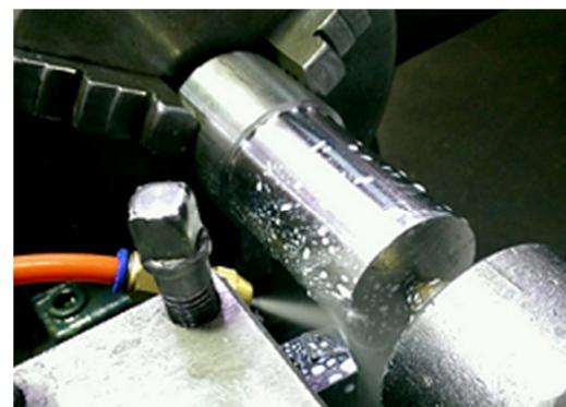
Fig. 2 Nozzle MQL, tool and workpiece setup
