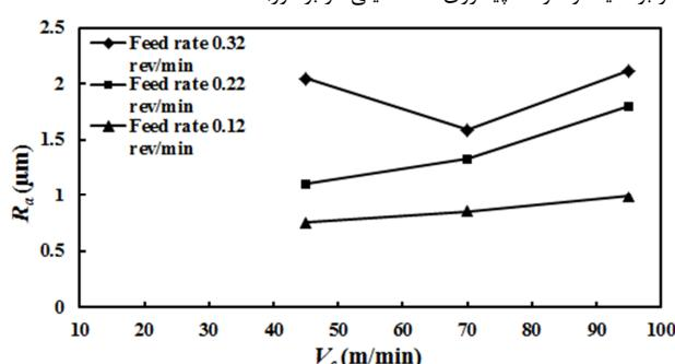
**Fig. 10** Effect of cutting speed on surface roughness for different feed rate under MQL conditions
