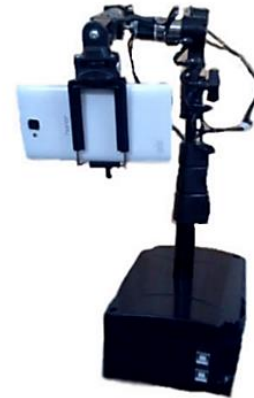
Fig. 5 The prototyped gimbal with 2-DOF
