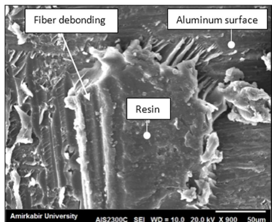
Fig. 22 SEM debonded surface image - fiber and resin breakage
