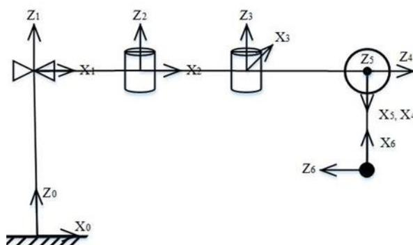
Fig. 2) The proposed system consists of 5 DOF and is a PRRRR mechanism (19).
