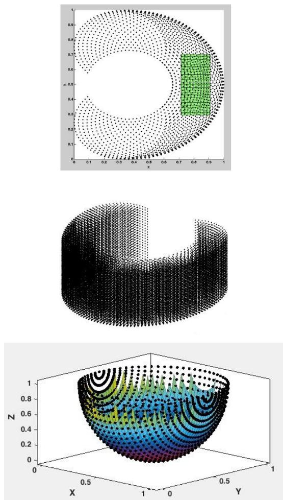
**Fig. 3)** (a) The actual workspace which is the rectangular area and the dexterous workspace which is the spotted area. (b) The vertical movement of the end-effector. (c) The normalized pathway of the end-effector.
