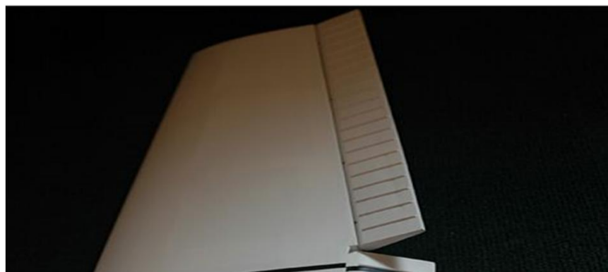
Fig. 3 Aileron lock at maximum deflection angle [13]
