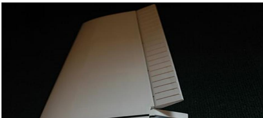
Fig. 3 Aileron lock at maximum deflection angle [13]
