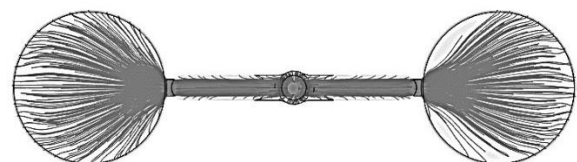
Fig. 3 Material flow at the filling time in 1 second
