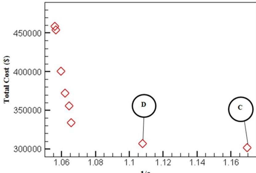
**Fig. 6** Pareto-optimal front for recuperator with counter-flow arrangement
