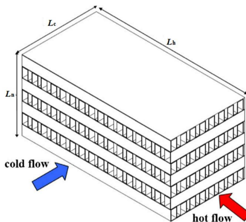
Fig. 2 Plate-fin heat exchanger with cross-flow arrangement [11]
