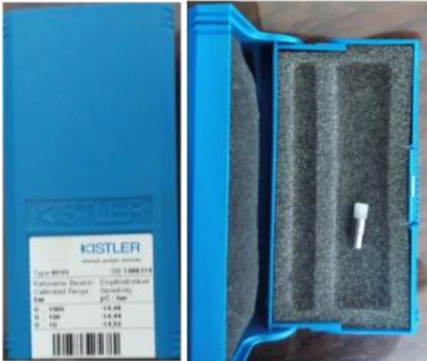
Fig. 4 A Sample of pressure sensor in test
