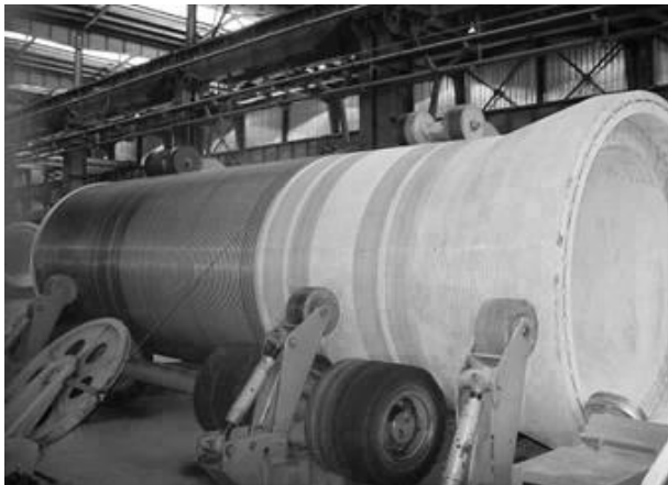
Fig. 5 Pre-stressing of concrete pipe with spiral rebar
