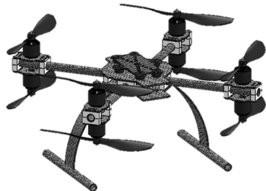
Fig. 1 Design of Mechanical Structure of Octorotor Flying Robot
