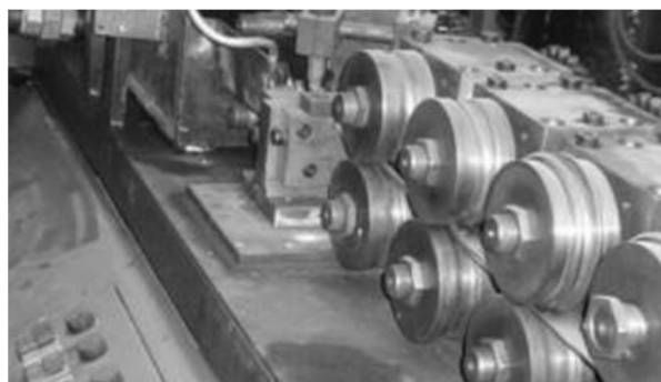
Fig. 3 A view of devices made for making the copper clad aluminum composite wire
