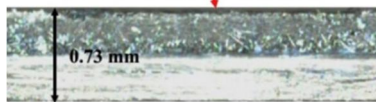
Fig.4 Typical images from optical microscopy of thickness of manufactured laminate with 50X magnification
