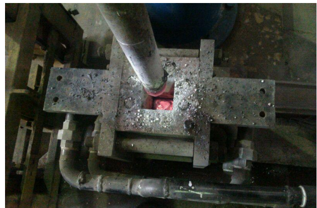
Fig. 2 Top view of mold immediately after the melting operation
