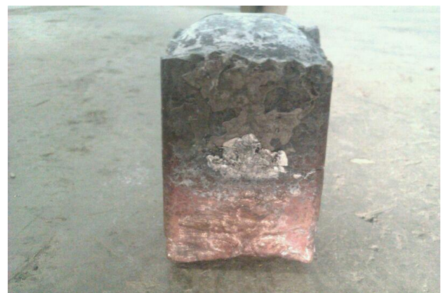
Fig. 3 Solidified copper-steel ingot
