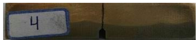
Fig. 4 A graded Copper-steel Specimen weakened by U-notch
