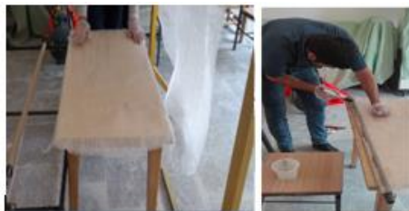
Fig. 5 Fiber winding and sample manufacturing
