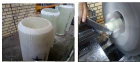
Fig. 7 chamfering the samples with a grinding machine
