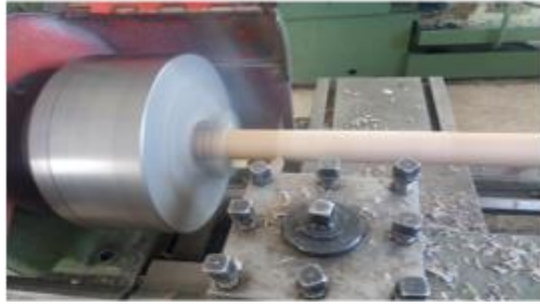
Fig. 4 Mandrel diameter correction with machining
