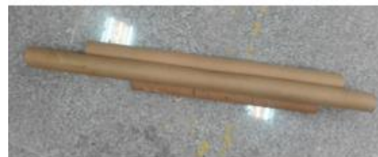
Fig. 3 paper mandrel for creating the composite tubes
