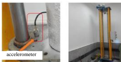
Fig. 9 Drop weight Device and accelerometer connected to it
