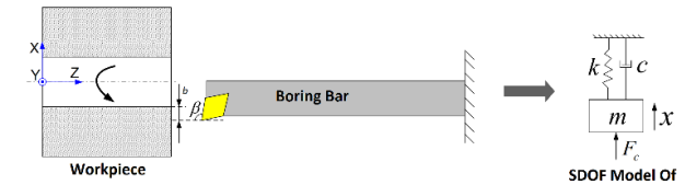
Fig. 2 A schematic of boring process
