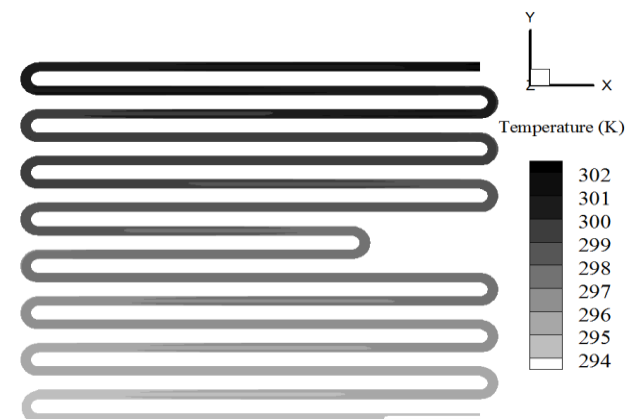
Fig. 9 Temperature variations of the fluid in the collector.
