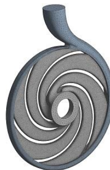
Fig. 3 Computational mesh for impeller and volute
