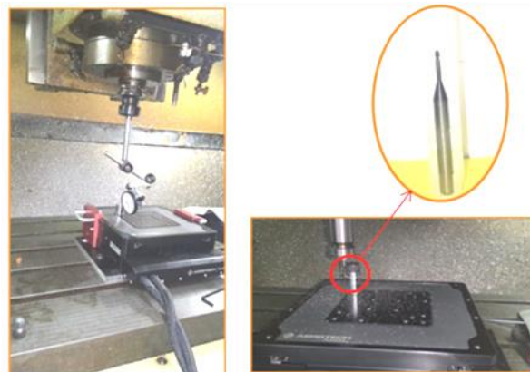
Fig. 13 Installation of the stage and fixture, and conducting machining experiments
