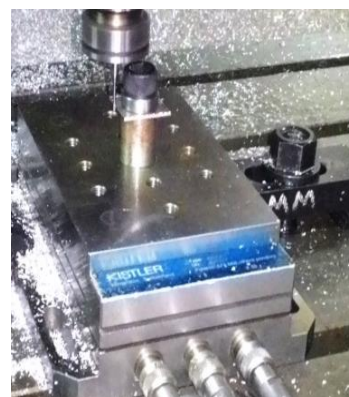
Fig.9 Measurement of cutting forces by a dynamometer
