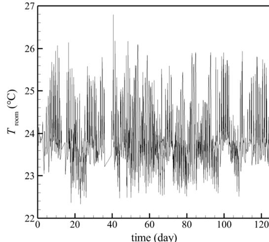
**Fig.7** variations of the room temperature building without insulation and with single glazings windwo for 123 days of cooling period
