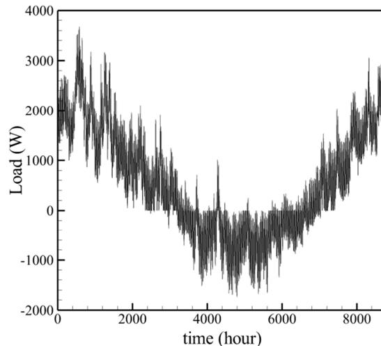
Fig.6 Hourly building loads for the building without insulation and with single glazings windows for 123 days of cooling period
