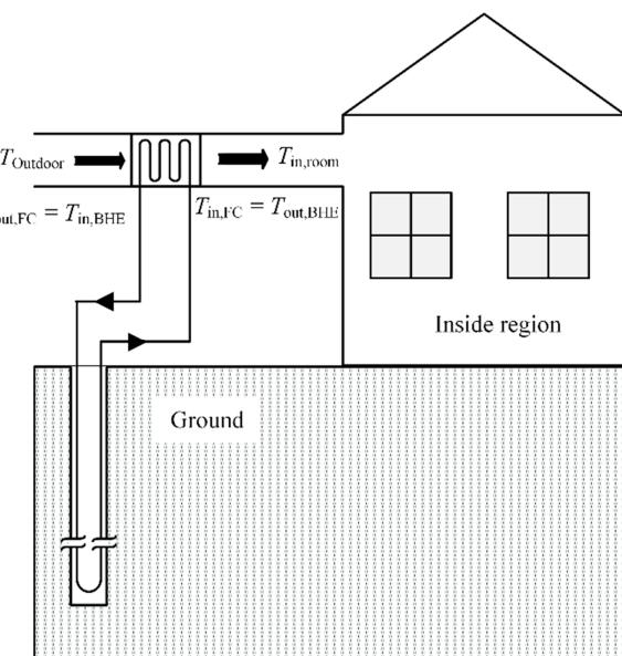
Fig.1 Schematic diagram of ground sink direct cooling system.
