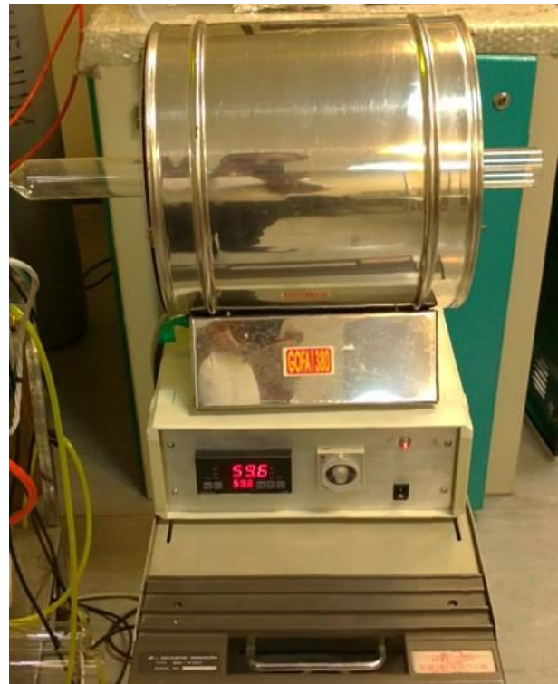
Fig. 3 Oxidation oven image
