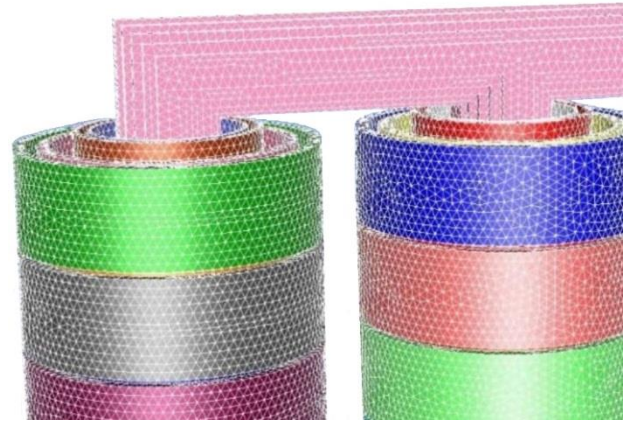
Fig. 14 Close view of transformer meshing
