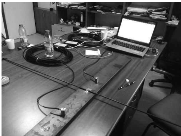
Fig. 7 Experimental sample for detection of attenuation
