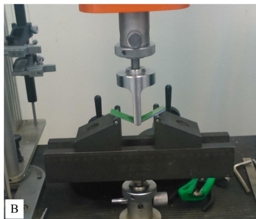
Fig. 5 A) Load-displacement diagrams of the three points bending test, B) the three points bending test setup
