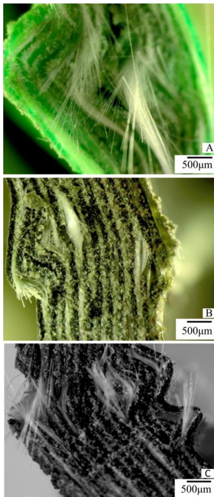
Fig. 8 Optical microscope images of the samples after three points bending test, A) Sample 1 produced at 160^{\circ}\text{C} , B) Sample 2 produced at 200^{\circ}\text{C} , C) Sample 3 produced at 230^{\circ}\text{C}
