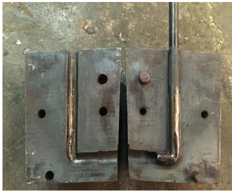
Fig. 2 Internal view of the used ECAP die
