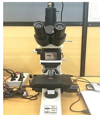
Fig. 5 Used device for measuring Vickers microhardness number
