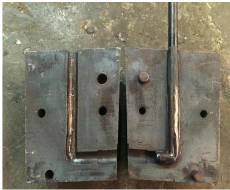
Fig. 2 Internal view of the used ECAP die
