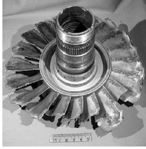
Fig. 2 Failed compressor blisk in the CT7-9B engine due to HCF [5]
