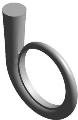
Fig. 2 Designed volute with CFTurbo software
