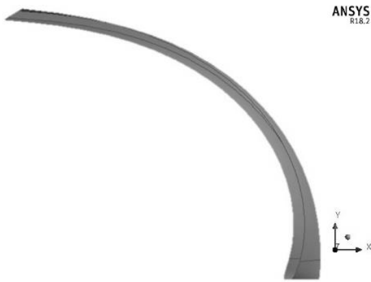
Fig. 15 The original blade of centrifugal pump
